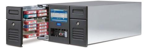
RLS-8350 is the entry level system for Qualstar's series of scalable midrange LTO libraries capable of storing over 12PB of compressed data in its largest configuration.
