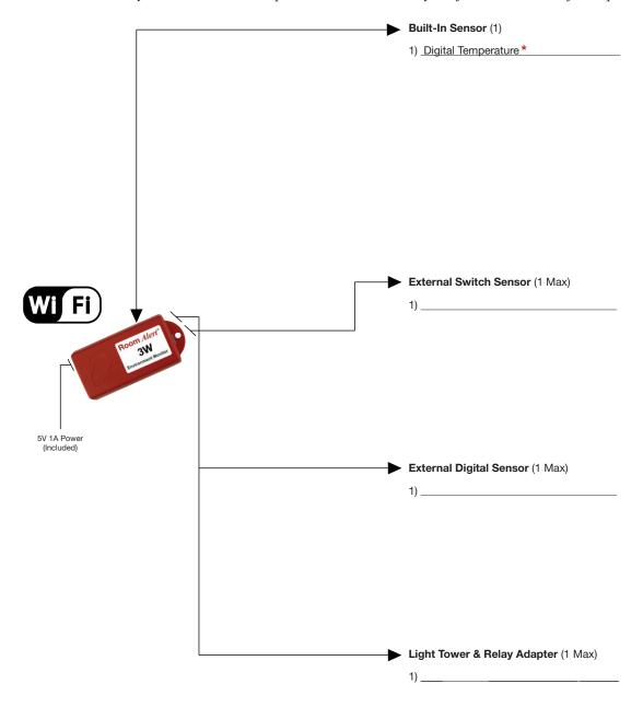
**Note:** The total sensor capacity of the Room Alert 3 Wi-Fi is 3+ sensors.
